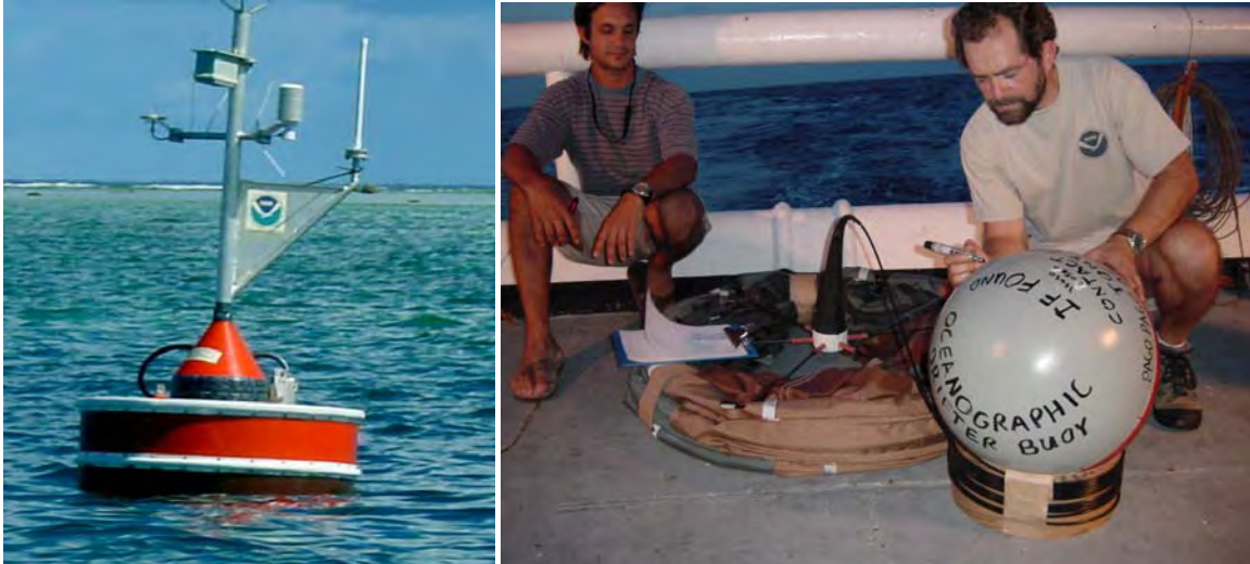
Figure 2: CREWS (Coral Reef Early Warning System) buoy deployed at Rose by CRED- left. The satellite telemetered buoy is anchored in the lagoon and records fine resolution data on climatic and ocean conditions. Drifter buoy being prepared for deployment near Rose by oceanographer Ron Hoeke and survey technician Phil White. Photographs: S. Holzwarth.
