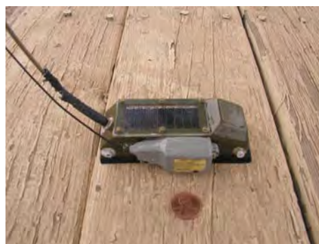
Figure 3. PTT GPS unit with VHF transmitter (gray) attached to the side. The whole unit weighs approximately 100 g.
