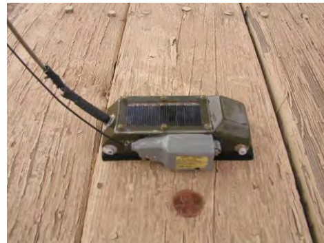
Figure 5. PTT GPS unit with VHF transmitter (gray) attached to the side. The whole unit weighs approximately 100 g.
