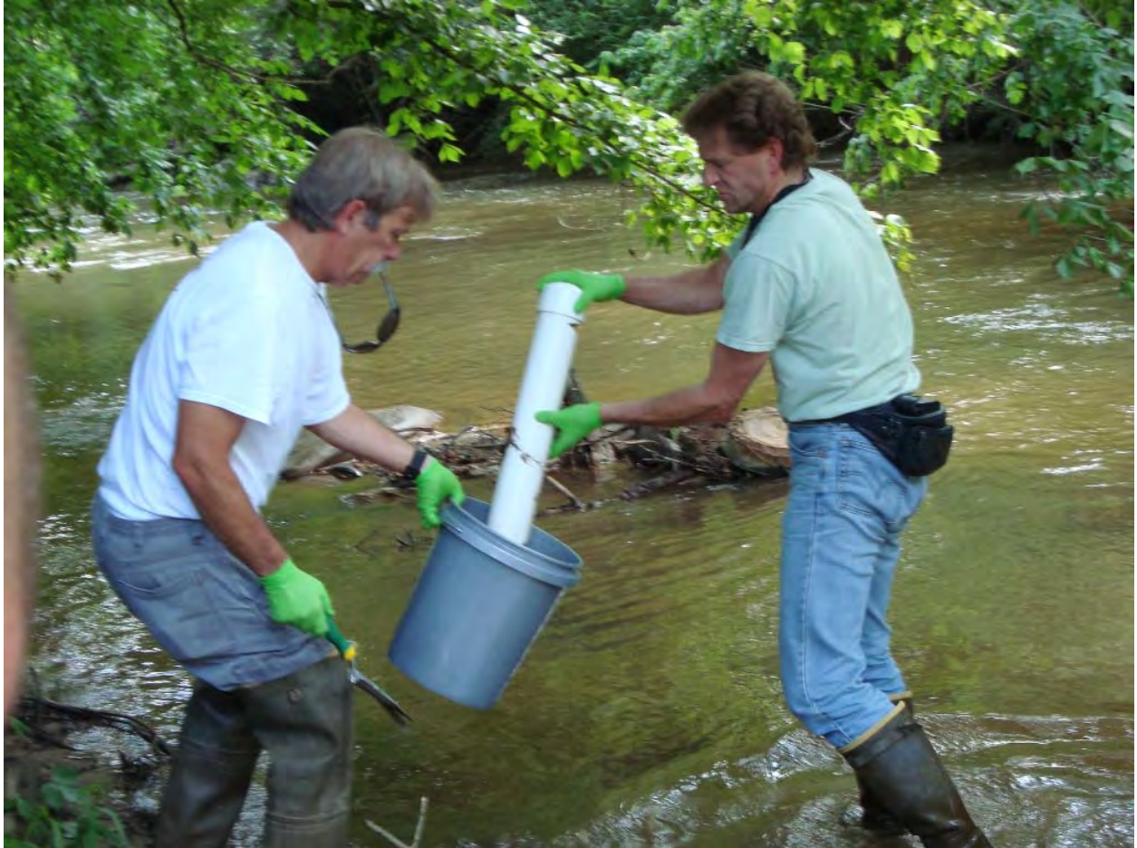
Photograph 3. Use of modified-Besser sampler.
