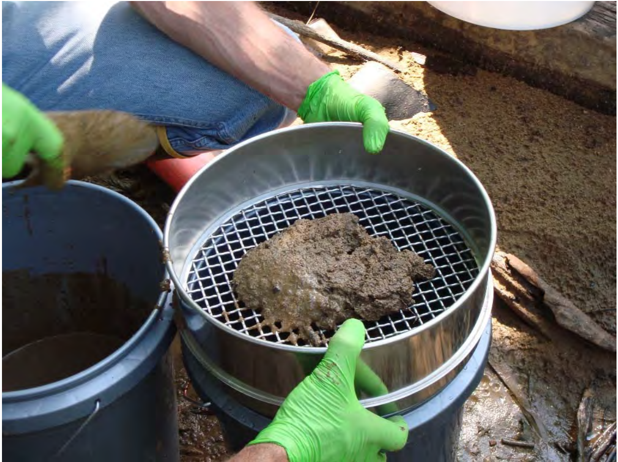
Photograph 5. Dry sieving of sediment through a 10 mm sieve.
