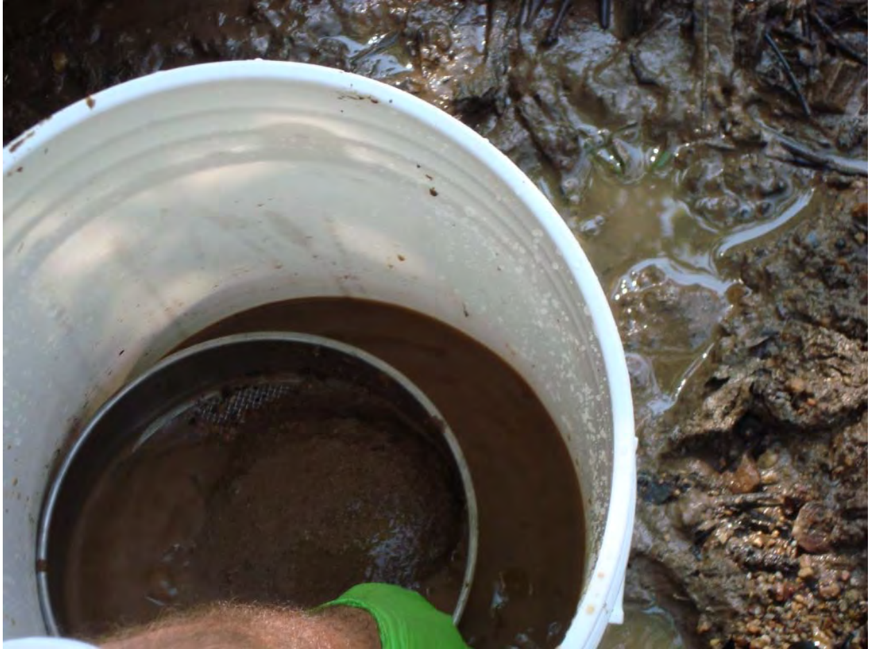
Photograph 8. Wet sieving of sediment through a 2 mm sieve.
