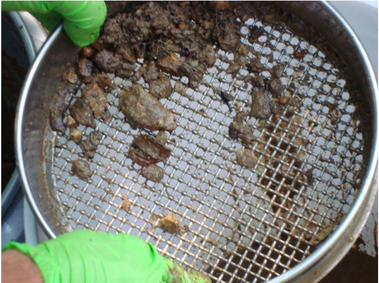
Photograph 6. Dry sieving of sediment through a 5 mm sieve.
