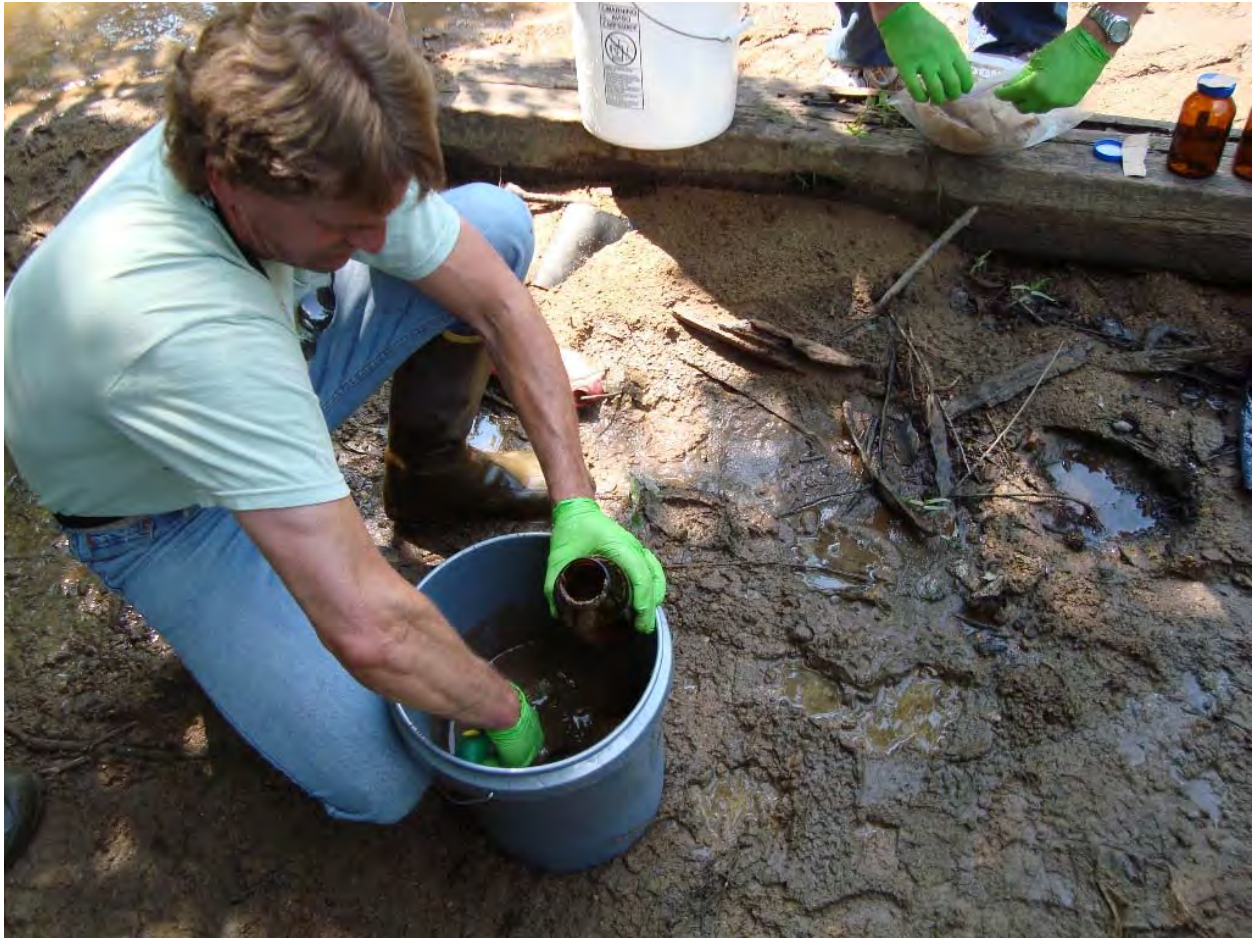
Photograph 4. Sampling of whole sediment composite.
