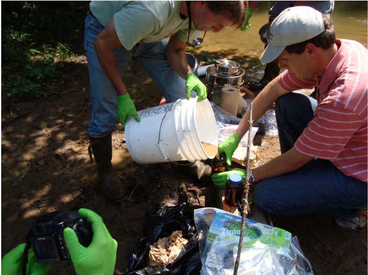
Photograph 9. Sample collection of overlying water from wet sieving of sediment.
