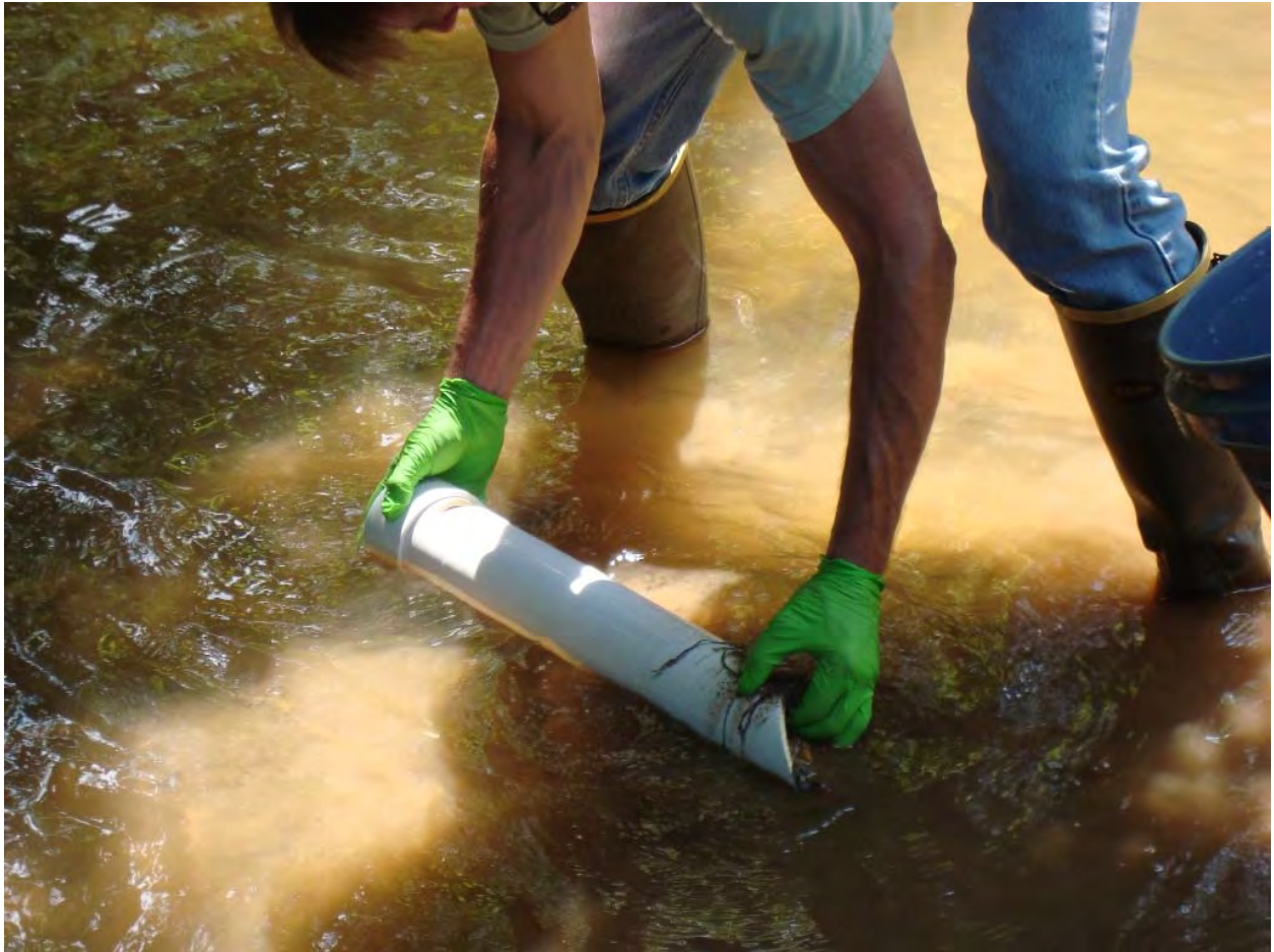
Photograph 2. Use of modified-Besser sampler.
