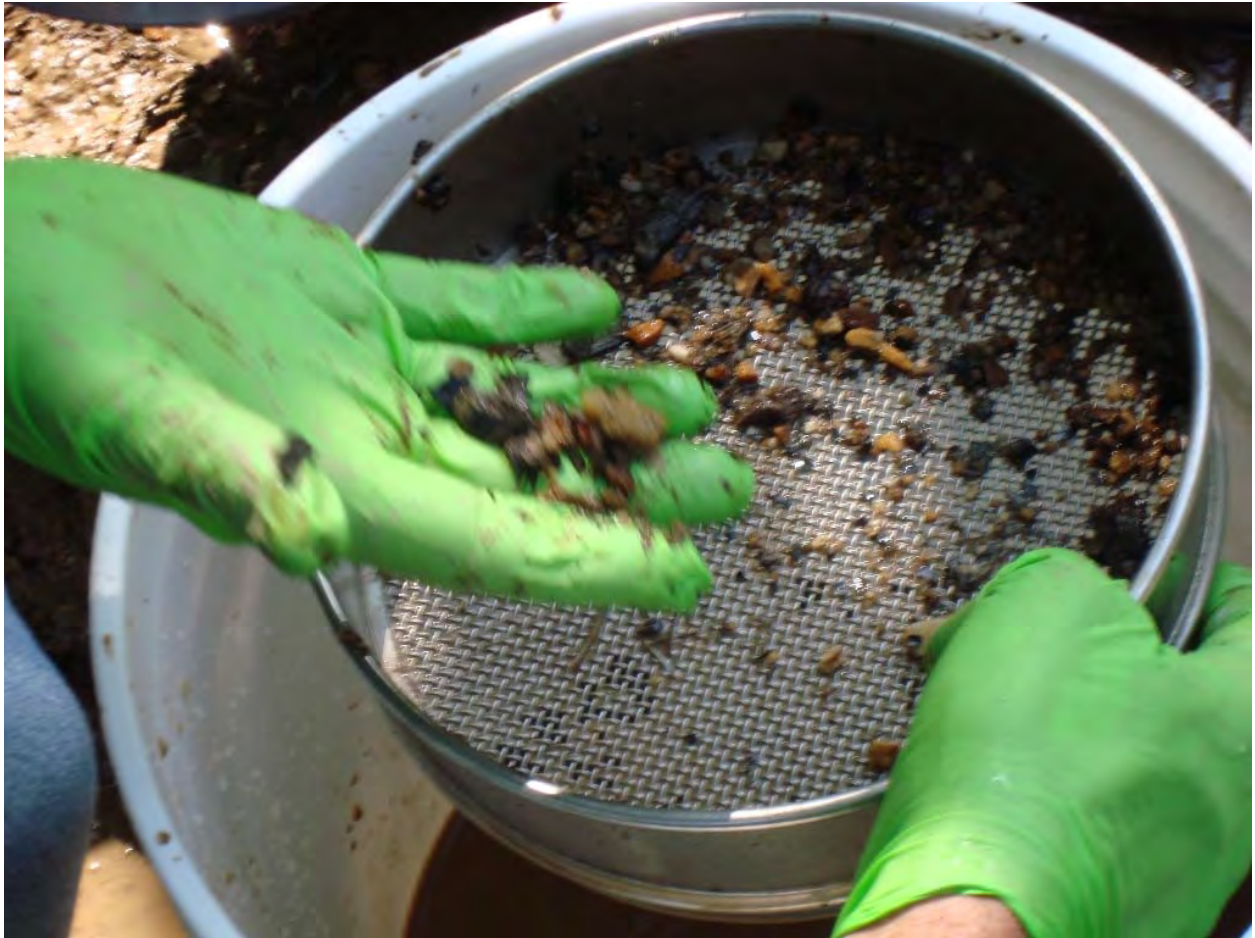
Photograph 7. Dry sieving of sediment through a 2 mm sieve.
