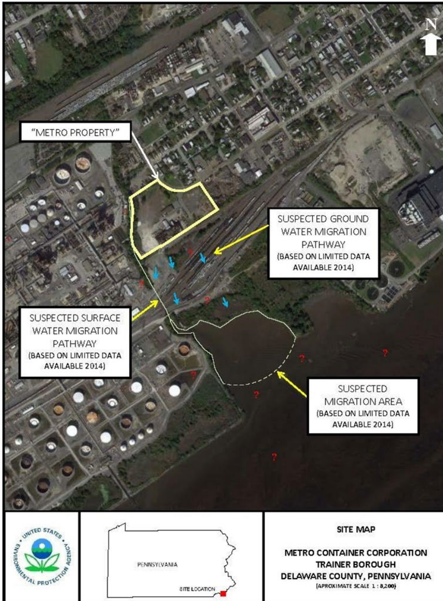
Figure 1. Metro Container Superfund Site Map. The “Metro Property” highlighted in yellow is the footprint of 10.4-acre Superfund Site with Stoney Creek (Suspected Surface Water Migration Pathway) denoted.
