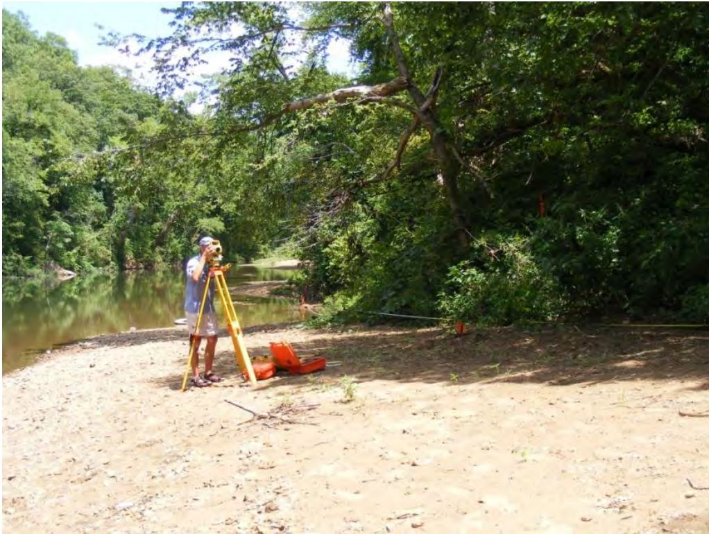
Surveying at Site #2 Bar. Notice survey tape and orange flags marking the 10m increment cross-section
