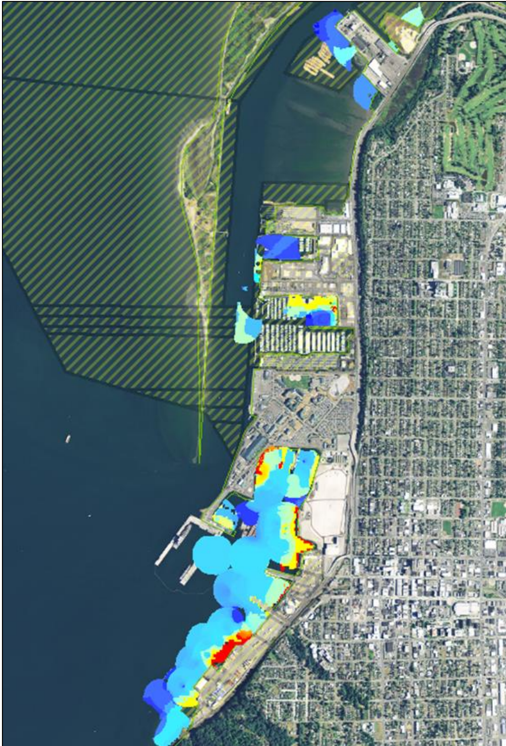
Figure 5. GIS map showing areas generated by combined map layers in the Habitat Equivalency Analysis (HEA), with greater injury represented by red and orange, and lower levels of injury represented by cool colors.
