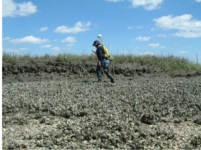
Figure 4. A Trimble® XP Pro GPS is used to determine the perimeter boundaries of each prospective restoration site prior to and following planting. This example of a two year old restored habitat in Two Sisters Creek, ACE Basin, SC was assessed to determine the area of vertical growth. Polygons are uploaded into ArcView and illustrated on GIS maps.
