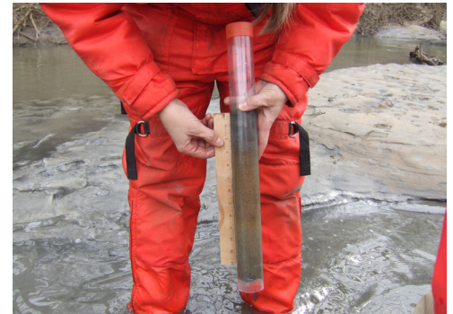
USFWS, Biologists completed in stream surveys to evaluate coal ash deposition over native river sediment.
