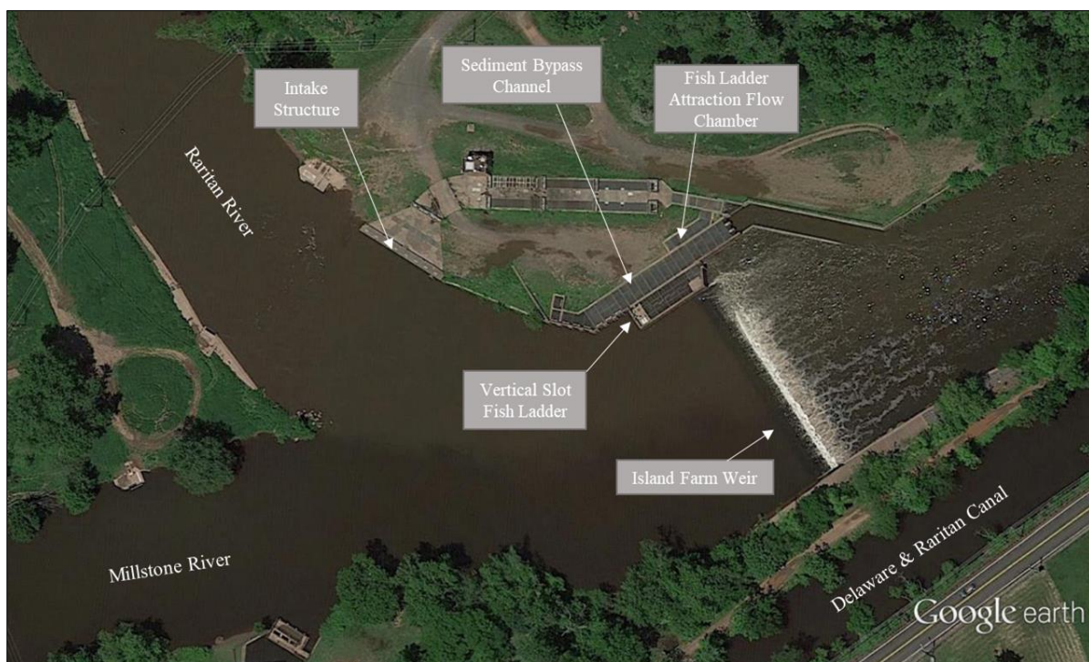
Figure 3. Island Farm Weir aerial view showing layout of major structures.
