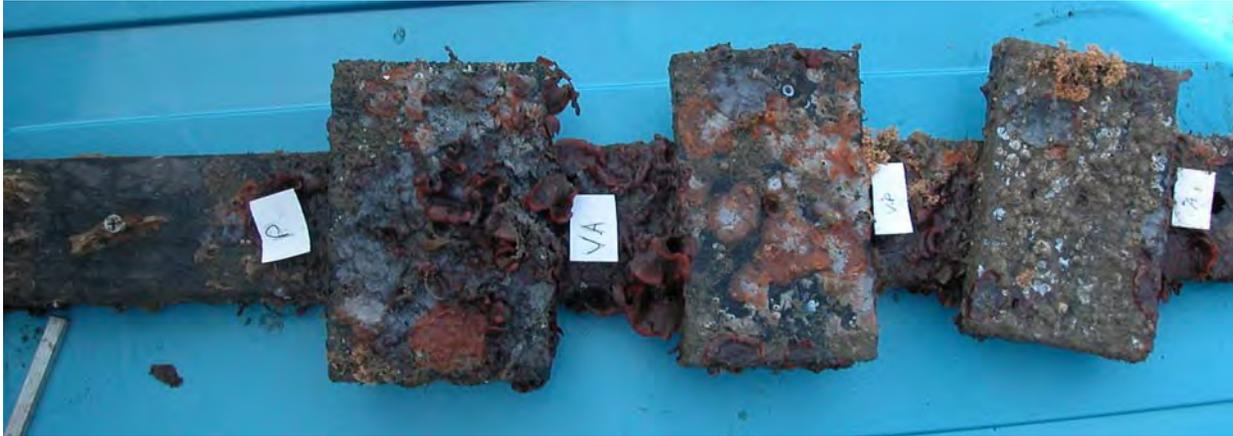
**Figure 3. Panel Array 1.** Panel treatments from left to right are uncoated ACZA-treated wood, vinyl-coated ACZA-treated wood, uncoated wood, and vinyl-coated wood. Most of the uncoated wood panel remains in place, but the surface has been eroded by minute wood-boring isopods called gribbles, exposing the much larger shipworm borings in some places and the white calcareous tubes that line shipworm borings in others.
