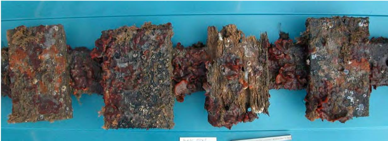
**Figure 4. Close-up of the untreated wood panel from Panel Array 1.** Surface removal by gribbles, and the shipworm borings and the white calcareous tubes that line shipworm borings (in a U-curve at upper right corner, near the center, and near the lower left corner) exposed by the gribbles can be clearly seen. Bryozoans and a few empty tests of barnacles are attached to the surface.
