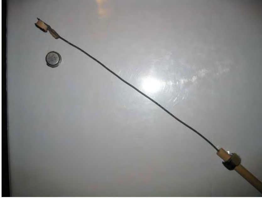
Figure 3. Temperature logger (iButton model 1922L; see arrow in photo) and assembled wand, to which an iButton was affixed (with velcro) and then inserted into artificial nest sites, to monitor attendance and visitation of Ashy Storm-Petrels at Orizaba Rock in 2010.
