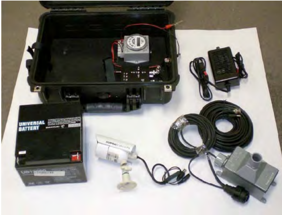
Figure A-1. Infrared camera components used to film Ashy Storm-Petrel behavior at Santa Cruz Island in 2010 (Photo by L. Halpin).
