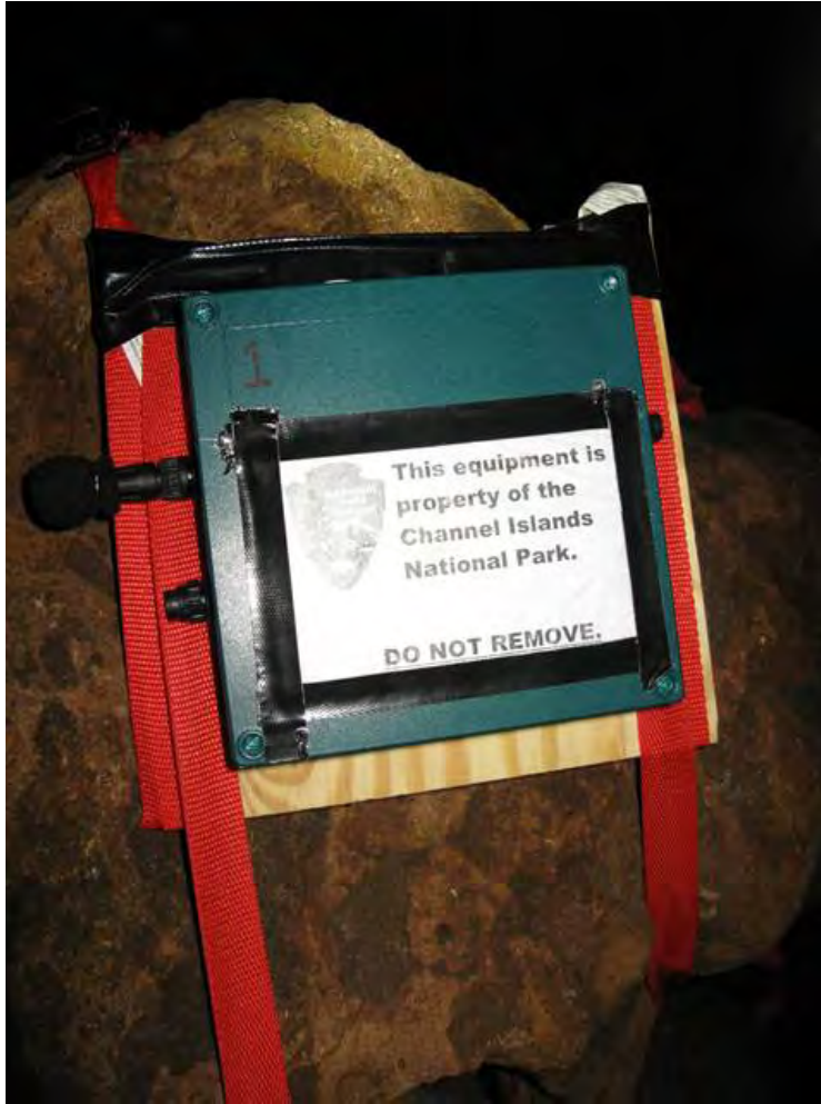
Figure A-3. Songmeter-2 Automated Recording Unit (ARU) at Cave of the Birds Eggs. (Photo by L. Halpin 2010)
