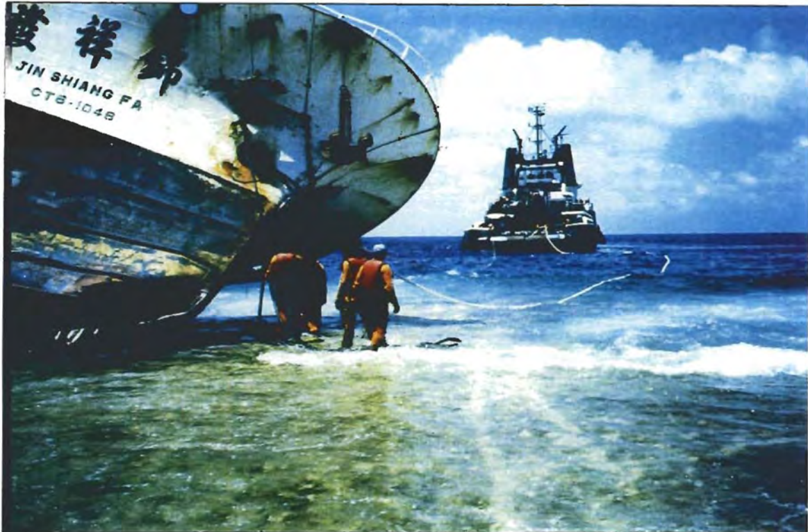
Figure 12 Salvage operation to remove the wreckage from the reef flat six weeks after the grounding.
