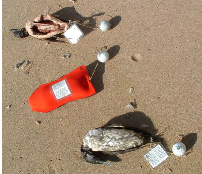
Figure 8. Different types of “carcasses” deployed in the rewash study. From top to bottom, carcass types are “eviscerated”, “dummy”, and “intact”. Transmitters are epoxied into foam floats connected by stiff metal rods. The laminated notices request that these units not be removed from the beach if found, and provide contact information.
