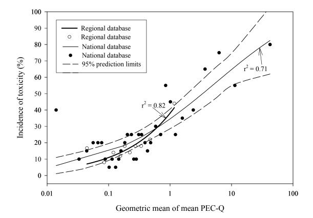
Figure 4.3. Relationship between the geometric mean of mean PEC-Qs and the incidence of chronic toxicity to amphipods (endpoints: survival only) in the national (28- to 42-day toxicity tests) and regional (28- to 42-day toxicity tests; n = 174, grouped by 15) databases.
